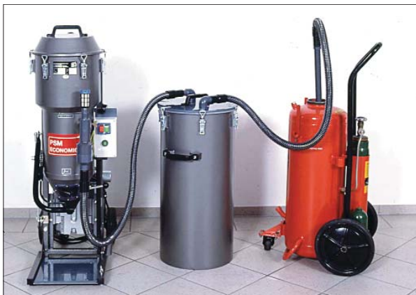
Fig. 3: During service work on 50 kg fire extinguishers, the fire extinguishing powder is first sucked from the portable fire extinguisher into the separate additional storage tank with the ECONOMIC.
