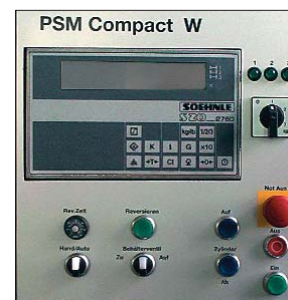
Fig. 3: Operating panel with all operating controls and integrated scales display.
