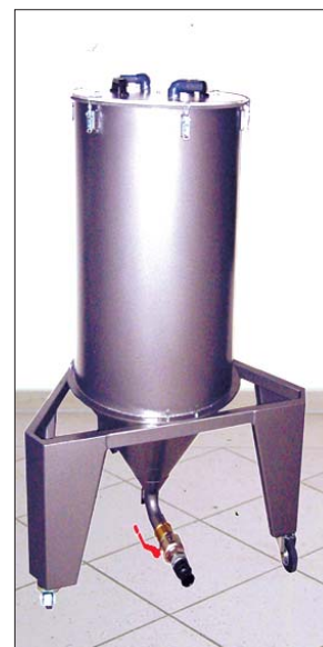
Fig. 7: Portable storage barrel for intermediate storage of 250 kg fire extinguishing powder. The removable lid has a 32 mm hose piece for connection with a powder suction machine. For removing powder, there is a connection with a closing ball valve and compressed air connection for loosening the fire extinguishing powder on the bottom of the silo.
