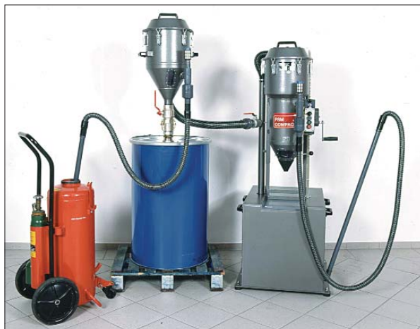
Fig. 4: The machine has a storage tank with a capacity of 12 kg. With an additional filter head (Fig. 6) portable fire extinguishers can also be serviced or filled with the PSM COMPACT S or fire extinguishing powder which is no longer fit for use can be removed from all fire extinguishers. The picture shows a 50 kg fire extinguisher being emptied.
