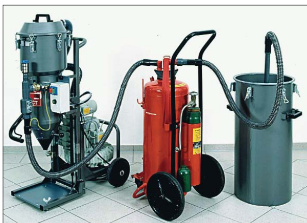
Fig. 4: After inspecting the fire extinguisher container, the SK 50 Set is attached and the fire extinguisher is refilled.
