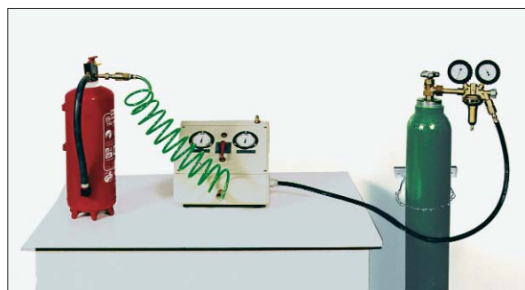
Fig. 2: Filling a sustained depression fire extinguisher from the nitrogen storage bottle.
