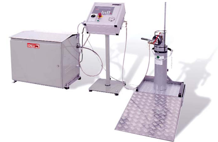
Fig. 1: The CFA 5 Carbon Dioxide Filling Unit is designed for the precise filling of CO 2 from the liquid phase. It is used to fill CO 2 bottles from 2 to 45 kg with frozen carbon dioxide from low-pressure tanks (15 to 20 bar).
