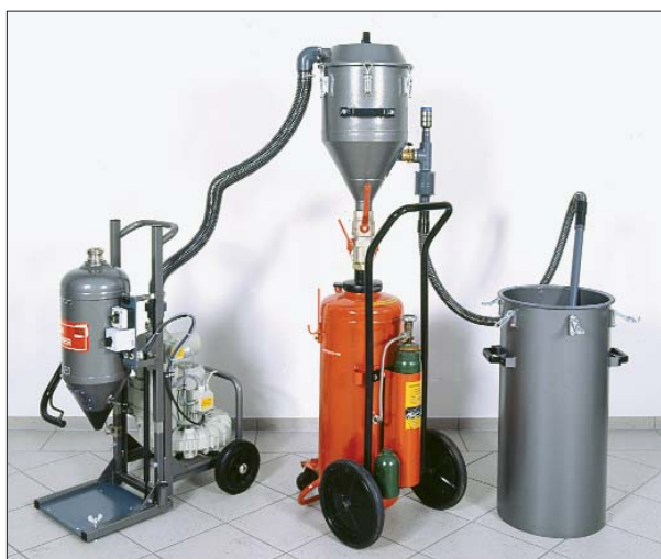
Fig. 4: With an adapter the filter head can be directly attached to portable fire extinguishers and these can then be filled from the 50 kg additional storage tank or a separate packing drum.
