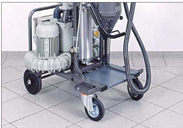
Fig. 3: The machine is fitted with 4 wheels for easy movement. The two front wheels are steerable and adjustable.
