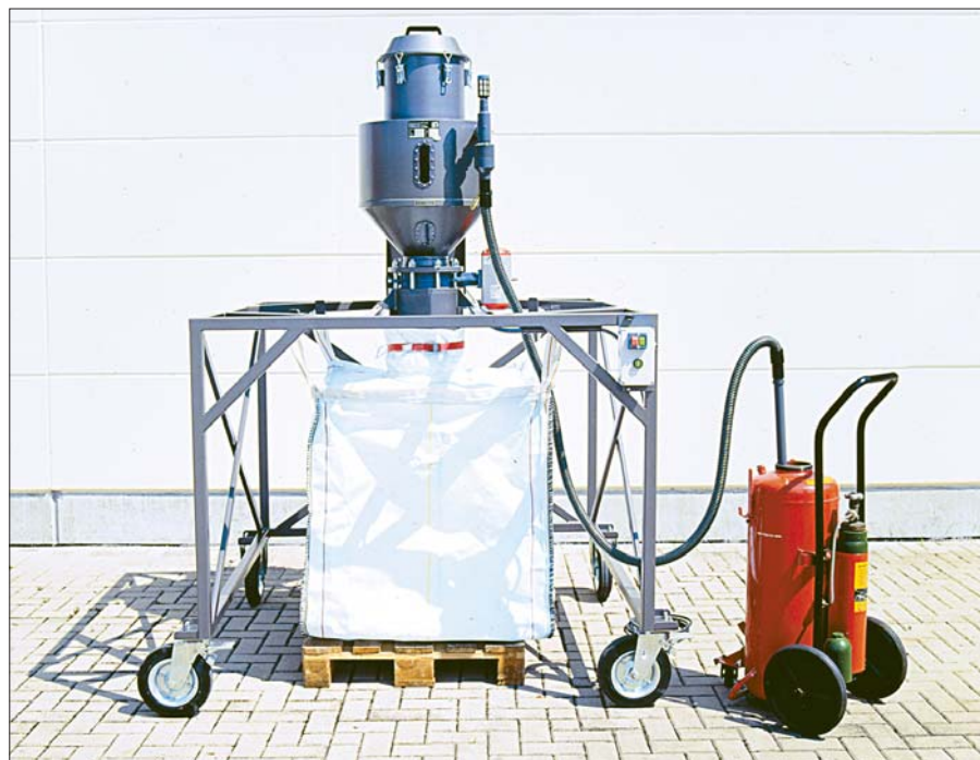
Fig. 1: With the PEA BIG-BAG the used powder from all fire extinguishers can be correctly disposed of. A special advantage is the mobility of the unit, so that the local conditions can always be taken into account despite the large capacity.
