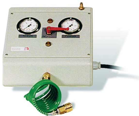
Fig. 1: With the SFA Nitrogen Filling Unit sustained depression fire extinguishers can be safely cushioned with nitrogen. The picture shows the unit with a connected N 2 spiral filling hose. The display of the admission pressure and filling pressure manometer is extremely precise.
