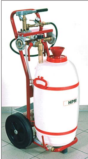
Fig. 4 and 5: With the HPM manual hydrant testing pump wall hydrants, rising mains and fire brigade pressure hoses can be tested with regard to pressure at rest and flow pressure.
