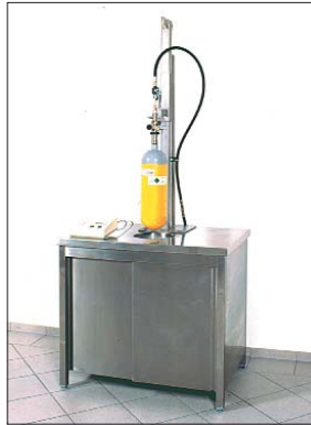
Fig. 7: The WJ 199 Water Jacket Testing Station is used to test the pressure of composite compressed gas bottles. The measuring principle of volumetric expansion is applied.
