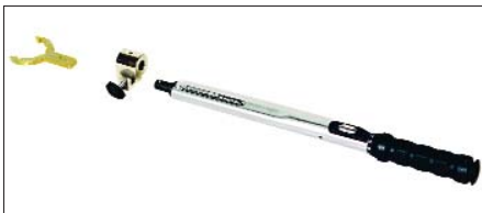
Fig. 2: Calibrated torque spanner for 20 - 200 Nm with an adapter for the special spanner for fire extinguisher fittings. This torque spanner has a test certificate according to DIN ISO 6789. As the lever lengths vary due to the differing lengths of the special spanners, a compensation table is enclosed, from which the appropriate corrections can be obtained without any difficulty. The adapters for attaching the special spanners can also be ordered individually. There are three different models for the standard torque spanners, so that a suitable adapter is always available.
