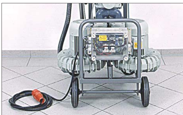
Fig. 2: A special sound absorber on the two electric motors ensures low operating noises. For smaller suction capacities the machine can also be operated with only one motor.
