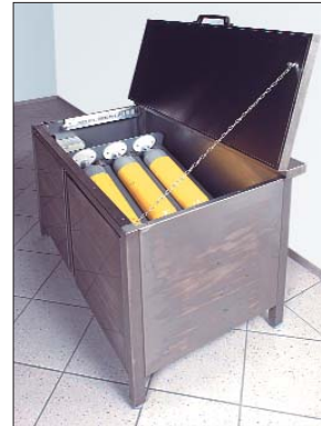
Fig. 8: With the tumbling device the inside of up to 3 compressed gas bottles can be cleaned simultaneously. It is enclosed in a special steel housing to deaden the noise.
