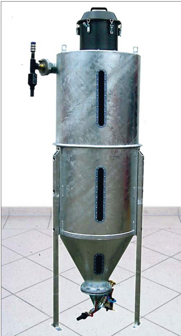
Fig. 4 and 5: Big Bag emptying funnel for supplying the PSM COMPACT A with fire extinguishing powder from a Big Bag. The emptying funnel is fitted with a manual powder valve, additional air supply with non-return valve and a sealable compressed air connection for additional ventilation. The front-opening safety supporting stand serves to secure the Big Bag should the loop break.
