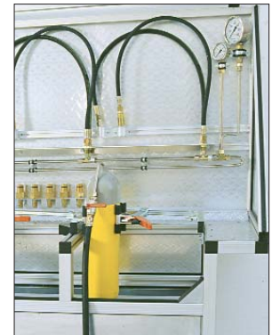
Fig. 5: Respiratory air bottle in the quick-change clamping device. Above it: the two high pressure hose connections for 500 or 60 bar maximum test pressure. On the right: the two test manometers for reading off the test pressure.
