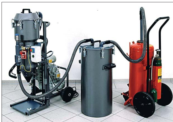
Fig. 3: By using a 50 or 250 kg additional storage tank, portable fire extinguishers can also be serviced with the PSM COMPACT. For service work on 50 kg fire extinguishers, for example, the fire extinguishing powder is first sucked out of the portable fire extinguisher into the separate additional storage tank.
