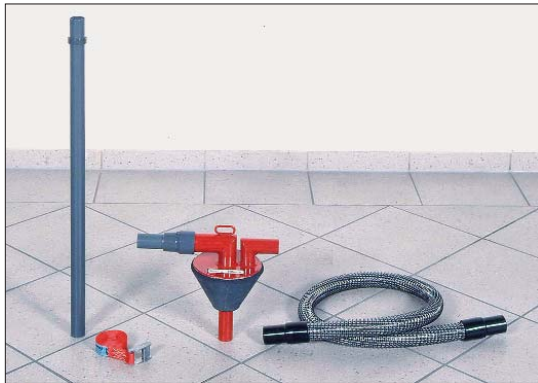
Fig. 7: To fill portable fire extinguishers – with the exception of the PSM POWER – the SK 50 Set is required, which is available as an accessory. It consists of an adapter with a sieve and clamp belt for the portable fire extinguisher, a 1.4 m-long suction hose and a 1 m-long suction pipe.
