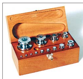
Fig. 5: Weight box with calibrated weights Class M3. Weight graduations: 1 to 2000 g.
