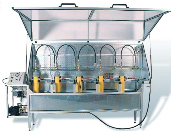
Fig. 1: Using the HTG 500 Hydrotesting Device steel or aluminium compressed gas bottles can be tested with an adjustable test pressure of up to 500 bar. The system guarantees maximum personal protection, as the water pressure test only releases minimal volume for pressure relief in the case of a rupture and, in addition, a shatter-proof Makrolon hood provides extra protection.
