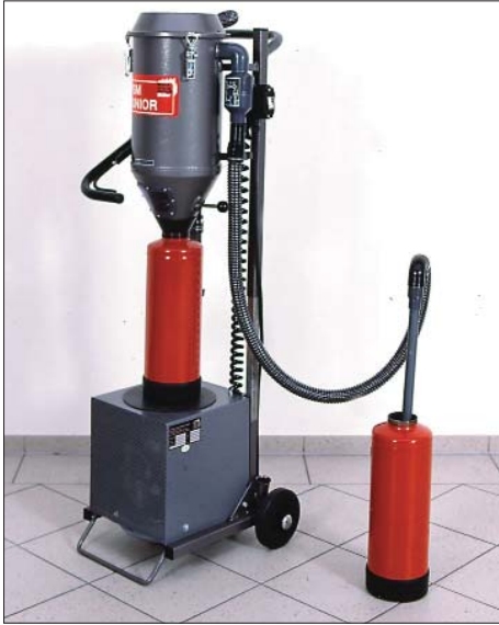
Fig. 5: If several fire extinguishers of the same type have to be serviced at the same time, the continuous method allows a time-saving batch service. Here two fire extinguishers are dealt with simultaneously: while one fire extinguisher is being emptied with the suction pipe, a second can be filled under the storage tank at the same time. (Picture example: PSM JUNIOR)
