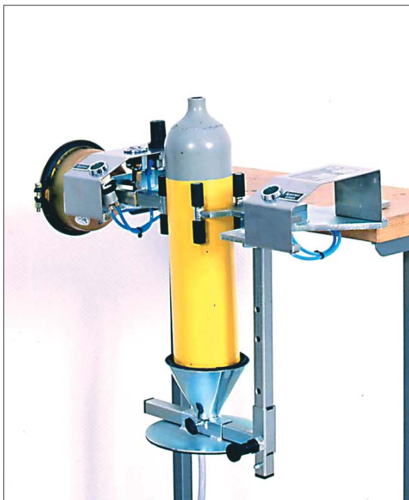
Fig. 5: The SVPA Clamping Device is suitable for quickly securing respiratory air device bottles and CO 2 bottles (2 and 6 kg). Carbon fibre composite bottles for respiratory air can also be clamped with special clamping jaws (accessory).
