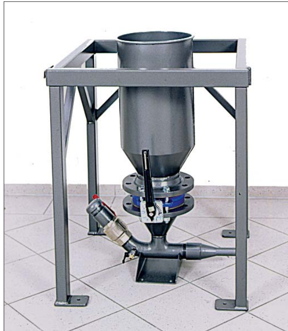
Fig. 4 and 5: Big Bag emptying funnel for supplying the PSM COMPACT A with fire extinguishing powder from a Big Bag. The emptying funnel is fitted with a manual powder valve, additional air supply with non-return valve and a sealable compressed air connection for additional ventilation. The front-opening safety supporting stand serves to secure the Big Bag should the loop break.
