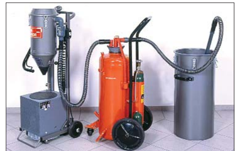
Fig. 5: With a 50 or 250 kg additional storage tank portable fire extinguishers can also be serviced with the PSM JUNIOR. The picture shows a 50 kg fire extinguisher being filled with the attached SK 50 Set.
