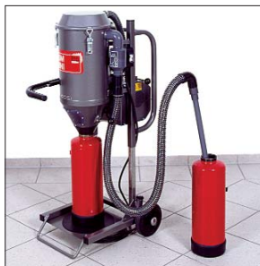
Fig. 3: If several fire extinguishers of the same type have to be serviced, two fire extinguishers can be handled simultaneously. While one fire extinguishing container is being emptied with the suction pipe, a second can be filled with the purified fire extinguishing powder under the storage tank at the same time.
