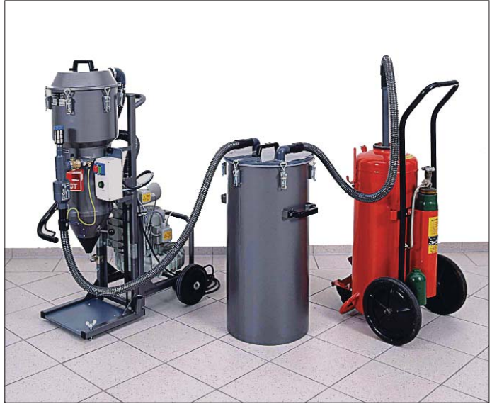
Fig. 6: During service work, the fire extinguishing powder from the portable fire extinguisher is first sucked into the separate additional storage tank. (Picture example: PSM COMPACT)
