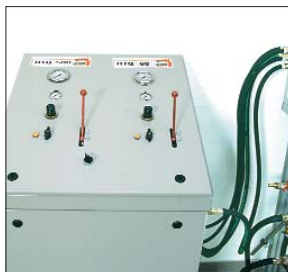
Fig. 3: The HTG 500/60 Hydrotesting Device is a combination of the HTG 500 and HTG 60 devices. It is therefore a device with all-round qualities that can be used to test all compressed gas bottles with the appropriate test pressure.
