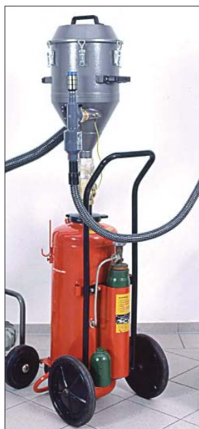
Fig. 4: The filter head opening can be closed with a ball valve. The filter head can then be removed by means of the quick action coupling and directly attached to all types of fire extinguishers using a supplied adapter.
