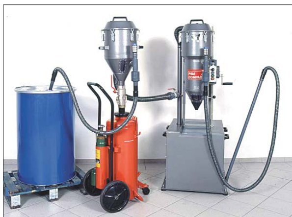
Fig. 5: After inspecting the portable fire extinguisher, the filter head (Fig. 6) is converted and the fire extinguisher is refilled from the barrel (Fig. 9) or the additional storage tank.
