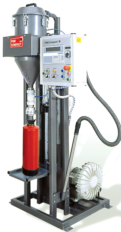
Fig. 2: The PSM COMPACT W is a stationary filling system for inspection services in a workshop and for large quantities. It is fitted with electronic scales that cut out automatically after reaching the filling quantity of fire extinguishing powder.
