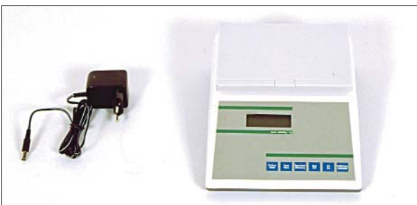
Fig. 3: Electronic scales with digital display up to 5000 g for CO 2 cartridges and CO 2 bottles. Battery or mains operated. Power supply unit comes as standard. Tare function. Numerical increment 1 g. Adjustable.
