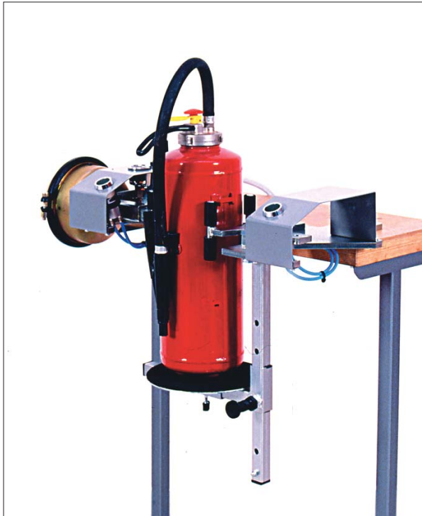
Fig. 3: The SVP Pneumatic Clamping Device is bolted on in front of the work bench. The supporting table for fire extinguishers from 2 to 12 kg is height-adjustable.
