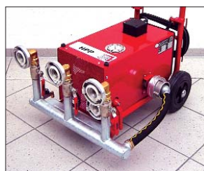
Fig. 3: A distribution battery is available as an accessory for testing up to 3 fire brigade pressure hoses simultaneously.
