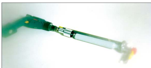
Fig. 5: The CO 2 cartridges of fire extinguishers can be screwed on and off with the screwing and unscrewing tool (see Tool No. 74) using a conventional hand drill. This is particularly helpful if the space is so limited that an open-jawed spanner no longer fits the hexagon nut.
