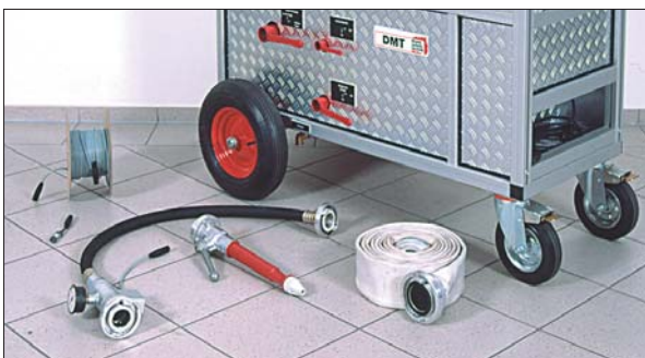
Fig. 2: A 5 m-long B pressure hose, a CM multi-purpose jet pipe with a special nozzle, a high pressure hose with manometer and sensor and a measuring cable come as standard.
