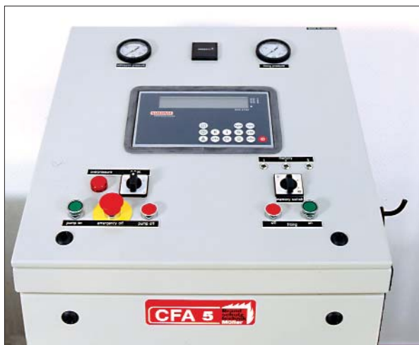
Fig. 3: The control stand is ergonomically designed to ensure comfort and convenience during operation. It contains displays for weight on the scales, filling pressure, circulating initial pressure, excess pressure control and an elapsed time meter. 3 different freely programmable cut-out weights can be called up for the scales with a selector switch.
