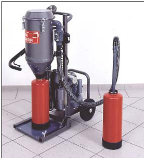
Fig. 3: With both the JUNIOR and the JUNIOR N two fire extinguishers of the same type can be handled simultaneously. While one is being emptied, the other can be filled with the purified powder from the storage tank.
