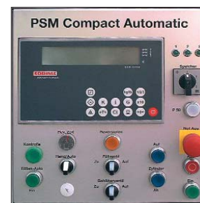
Fig. 3: Operating panel with all operational controls and integrated scales display.
