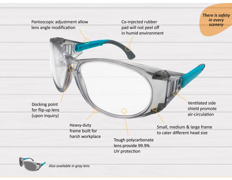
Caring ICARO. The compationate eyewear for you. With a well ventilated side shield and a docking point for flip-up lens. This versatile eyewear allows user to adopt in any kind of workplace, indoor or outdoor. It is well suited for workers who are exposed on harsh environment. ICARO have a tough lens highly recommended if workers will be exposed on chemical splashes.
